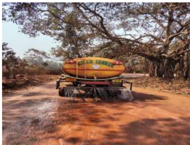
Photo-6 Water sprinkling through mobile tanker on mineral transport road adjacent to mines lease.
