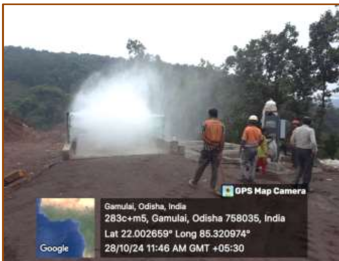
Photo-3 Wheel wash facility at the exit gate of Mines with recirculation system
